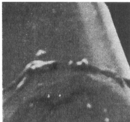
FIGURE 12 Scanning electron micrograph of portion of pulled out glass rod.
